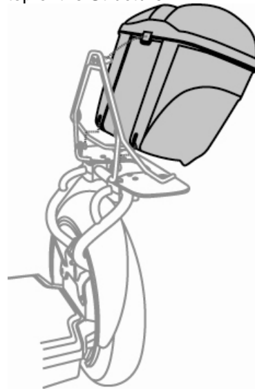
Figure 6. Positioning the Hard Side Case for installation.
