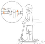
Release the accelerator and the kinetic energy recovery system (KERS) initiates automatically to brake slowly; squeeze the brake lever for a sudden brake.
