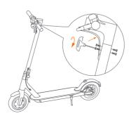
2. Install the handlebar onto the stem.
