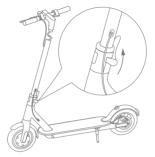
3. Use the hexagon wrench in the packaging box to lock the screws on both sides tightly
