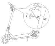
2. Install the horizontal handle on the vertical tube
