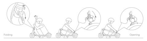
Confirm that the electric scooter is off; hold the vertical tube and push aside the folding thumb shifter, open the folding wrench, and hook the tinkle bell with back mud guard after aligning the position of tinkle bell and back mud guard. For opening the electric scooter, press the hook at the tinkle bell place, when the hood of tinkle bell is divorced from hook of mud guard, stand the vertical tube, lock the folding board tightly and put the folding thumb shifter back.
