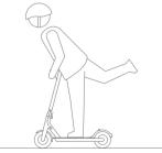
$\triangle$ Do not step only one leg on the pedal when the scooter is running
