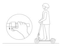
3 Step on the pedal by both legs when the electric scooter is gliding on the ground, and slightly press the accelerator thumb shifter (the accelerator can be started when the speed is over 5km/h)
