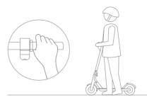
Do not press accelerator thumb shifter when pushing the scooter for walking
